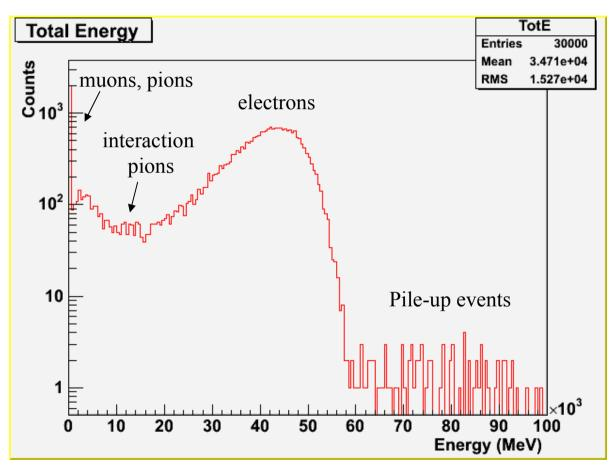
For tertiary beams ( $E \le 50$  GeV), only mixed beams are available: Similar number of pions and electrons.
