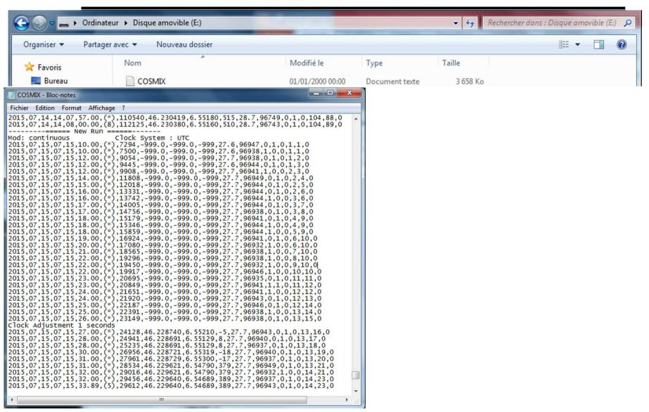
y, mo, d, hr, min, s, (GPS sat.), Ton\*(1/100 s), long, lat, alt (m), T(°C), P(Pa), Tr1, Tr2, Tr1∩Tr2, C1, C2, C1∩C2 \* time lapse since powered on
