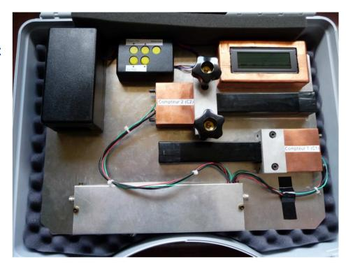
Counting and data logging via arduino and SD card
