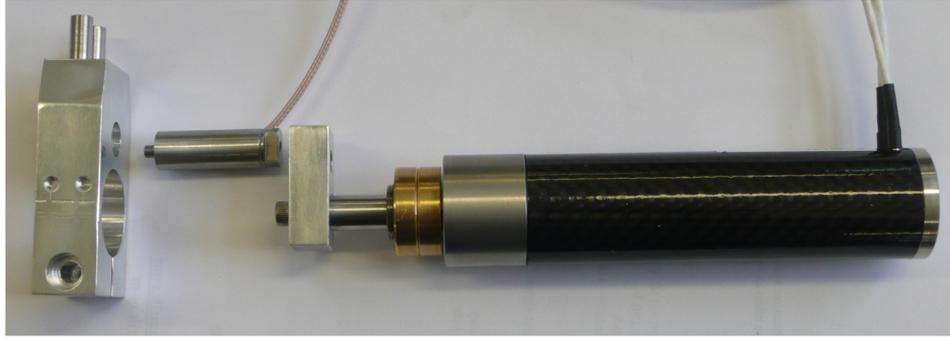
**FIGURE 2.** The new low-voltage stepper motor and piezo actuator, along with supports, being used in the DPUNS device.
