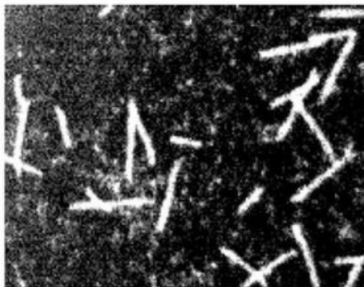
FIGURE 3.18 Superimposed proton–triton tracks obtained with an exposure time of 1 s with a CCD readout of a GEM-based neutron detector. (From Fraga et al., 2002. Reprinted with Permission from Elsevier © 2002)
