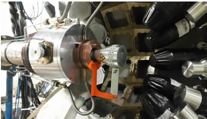
Figure 2 The nu-ball array coupled to the LICORNE neutron source. The ^{232}\text{Th} high-mass, low-density target can be seen in the centre.
