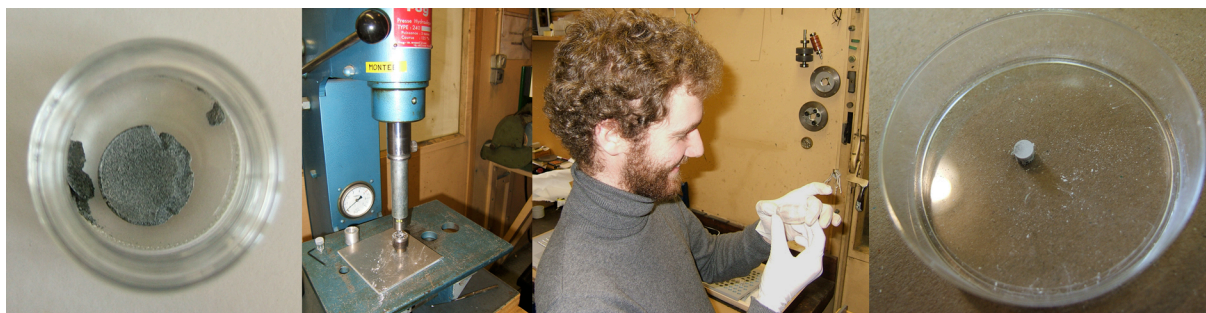
Figure 13: Pellet preparation from reduced \text{TiO}_2 in 2008
