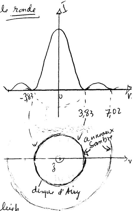
[A.N./TD] D4 :  $f = 10^2 \text{ mm}$   $\lambda = 0,55 \mu\text{m}$   $2R = 0,1 \text{ mm} \Rightarrow x_{\min} = 0,67 \mu\text{m}$
