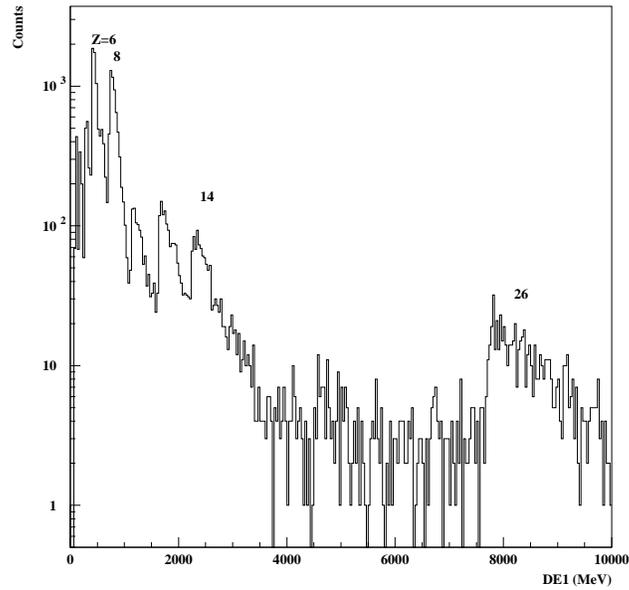
Figure 2 Expected distribution of ionisation energy deposited by the cosmic-ray ions in one CsI crystal. The main peaks are labeled according to the ion atomic numbers.
