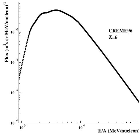
Figure 1. Energy spectrum of carbon ions at GLAST's flight altitude, as calculated with CREME.
