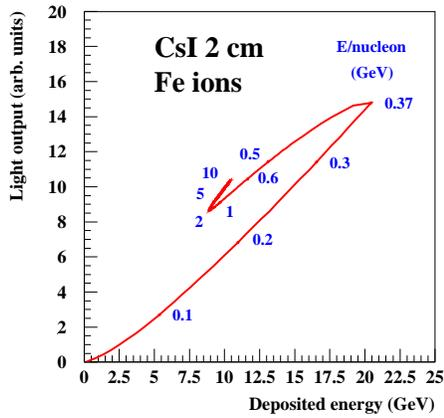
Figure 4. Possible  $L(E)$  for Fe ions in a 2cm-thick CsI crystal.
