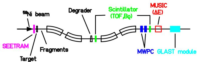
Figure 7. Sketch of the proposed experimental setup.
