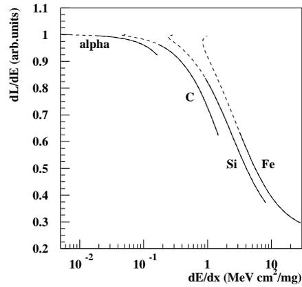
Figure 5. Calculated  $dL/dE$  as a function of  $dE/dx$  for four different ions, using the functions of ref.[9].
