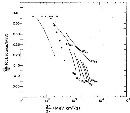
Figure 6. Compilation of experimental  $dL/dE(dE/dx)$  for different ions in NaI. The open (solid) symbols and dashed curve correspond to H (He).
