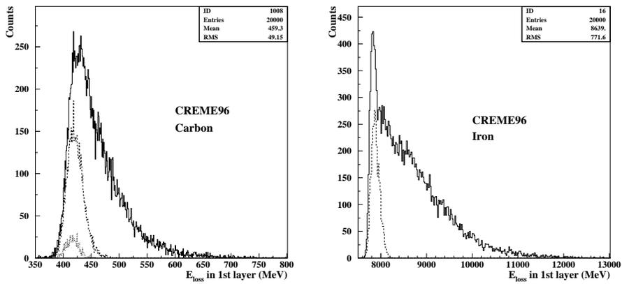
Figure 3. Distributions of ionisation-energy for carbon (left) and iron (right) ions. The dashed histograms correspond to the distributions resulting from a filtering procedure.
