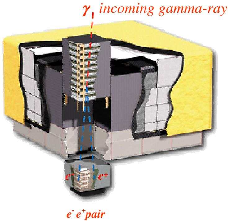
Figure 1 Sketch of the Fermi-LAT. The telescope comprises 16 towers, composed each of a tracker (upper part) and a calorimeter (lower part). An anticoincidence system (tiles in light gray) encloses the upper part and is covered with a micrometeorite shield (in yellow).
