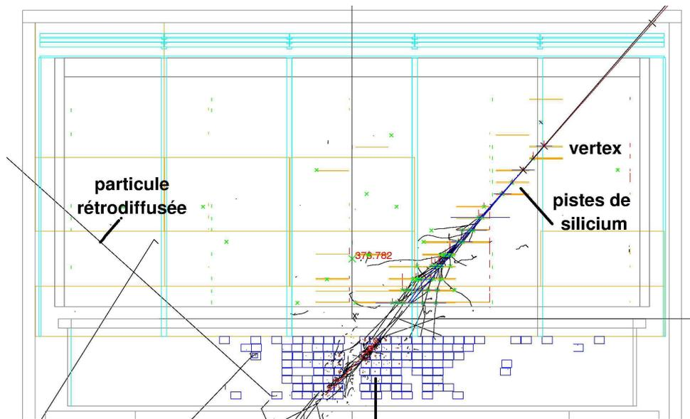
Figure 2 Result of a simulation showing the detection of a 5 GeV photon detected by the LAT.
