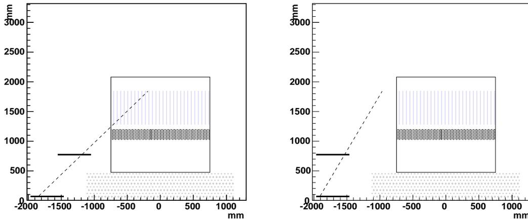
Figure 2: Muon telescope placement. Left: for run 77013003, with the top scintillator unbolted from the stand. Right: for runs '947, '948, '970. No coincidences were observed in data taken in this configuration.
