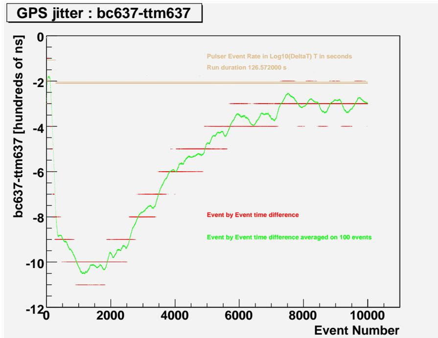
Figure 3: Differences in the times recorded with two independent VME GPS modules, a bc637 and a TTM637, both from Symmetricom, a few days prior to the first runs at the Factory of the Future. The former used a Trimble antenna, the latter interprets the GPS L1 signals on the VME board. Time agreement improved from 1  $\mu$ s to 0.3  $\mu$ s over the 2 minute data run.
