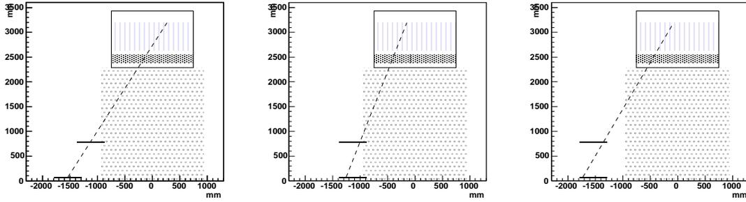
Figure 7: LAT integrated with spacecraft, mounted on stand. Left: top scintillator unbolting from the stand and moved closer to LAT, as in November tests. Middle: Both scintillators unbolting and moved closer. Right: Both paddles fixed in original position on stand. The dashed lines illustrate muon tracks striking the scintillator edges at  $\frac{1}{2}$ ,  $\frac{1}{4}$  and  $\frac{1}{8}$  of the paddle width from the paddle edge, respectively, for the 3 frames.
