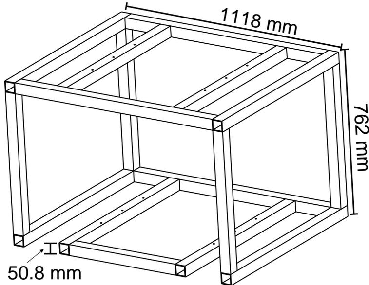
Figure 1: The scintillator paddle support stand for the muon telescope. Three screw-holes for the paddle support brackets are visible on four cross members. The phototube axes run parallel to the lines of holes, half-way between the cross members. The phototube bases extend beyond the long edge of the stand, hence the left-most (East) edge of the stand is placed next to the LAT. The top paddle is moved to extend beyond the left-most edge. Adapted from [10].
