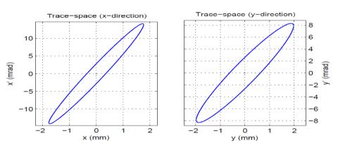
Emittance measurement in the range of  $5\pi$  mmmrad, higher than specs but the measurement is not reliable (see problems)
