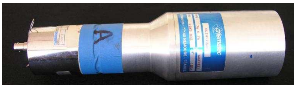
NaI detector for prompt fission \gamma . CIEMAT
