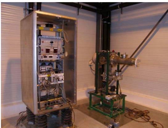
Figure 6: (a, left) FEBIAD ion source and part of the HV platform installed at the CENBG. (b, right) Representation of the steerers + quadrupole at the exit of the ion source within the code SIMION.
