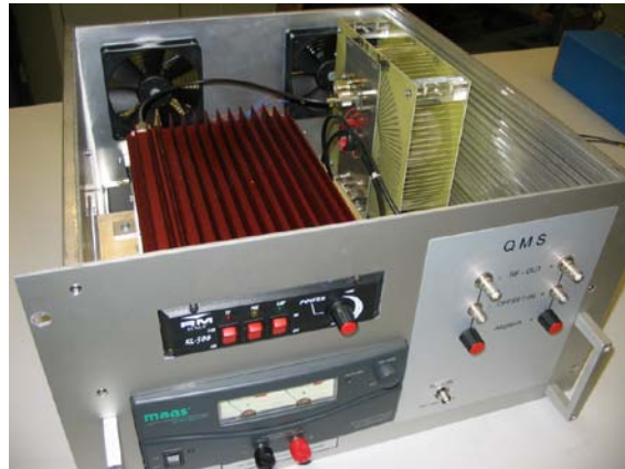
Fig. 6: Left: QMS and diagnostics unit, right: customized RF amplifier designed to provide RF amplitudes up to \sim 1800 V_{pp} .
