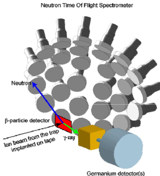
**Figure 31:** CIEMAT nTOF spectrometer setup as it will be used at IGISOL- Jyväskylä.
