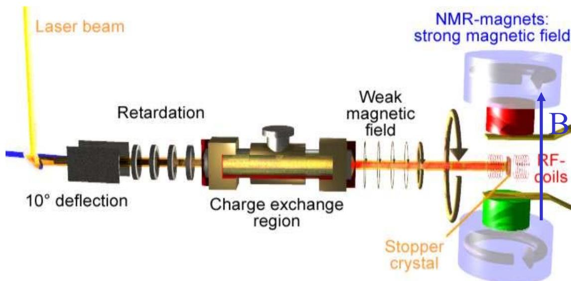
**Figure 20:** Schematic layout of the experimental setup for collinear laser spectroscopy and  $\beta$ -NMR on atom beams.
