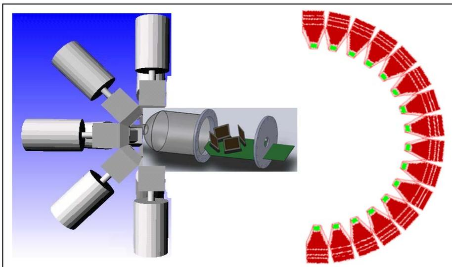
**Figure 37:** Schematic view of a possible decay experiment setup. A  $2\pi$   $\gamma$  array is surrounding a versatile charge particle detector setup. In forward direction, a ToF neutron wall can be added.
