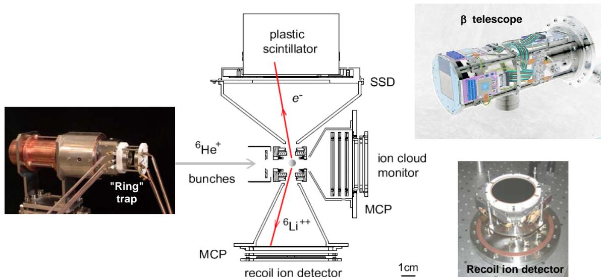
**Figure 48:** Details of the transparent Paul trap surrounded by suitable counters to detect the products from the  $\beta$  decay of ions in the trap.
