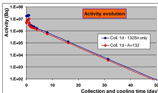
**Figure A6:** Activity evolution for the simulated experiments ( $^{132}\text{Sn}$  and  $A=132$ ).
