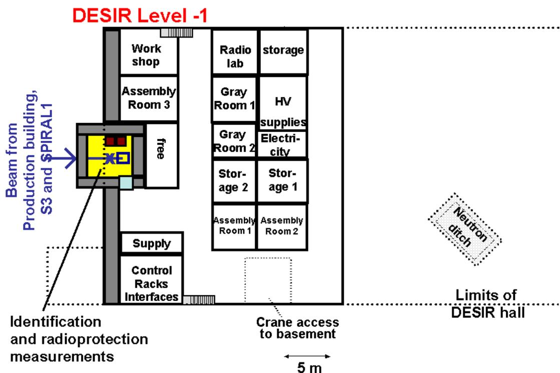
*Figure 7: Possible arrangement of the different technical rooms of DESIR, most likely in the basement of the DESIR hall.*
