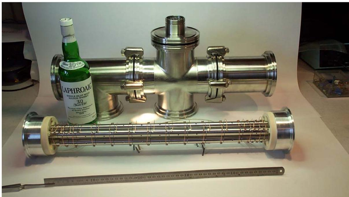
**Figure 17:** Photograph of the segmented quadrupole linear ion trap. The overall length of the quadrupole structure is about 50 cm [COLETTE]. Also shown is the gas bottle.
