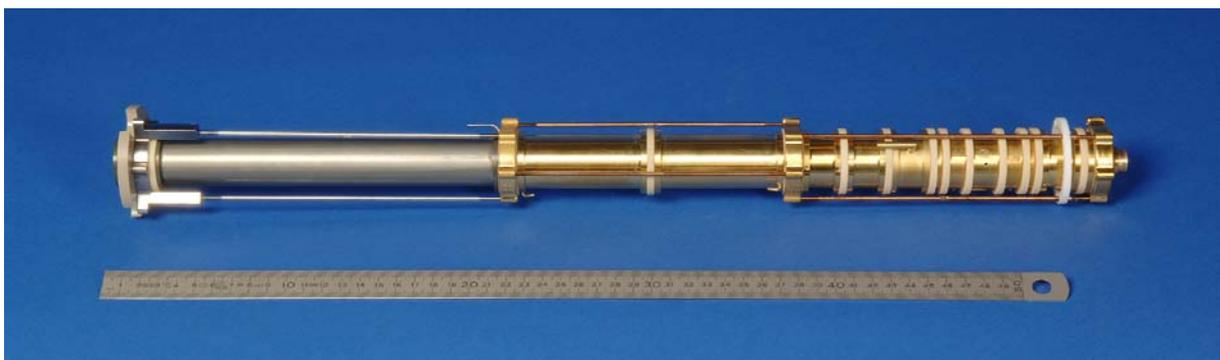
*Figure 25: Cylindrical Penning trap system. The Penning trap is situated at the right end of the figure. The system proposed will contain two such cylindrical Penning traps like the TRIGATRAP shown in the photo (G. Otto, GSI).*
