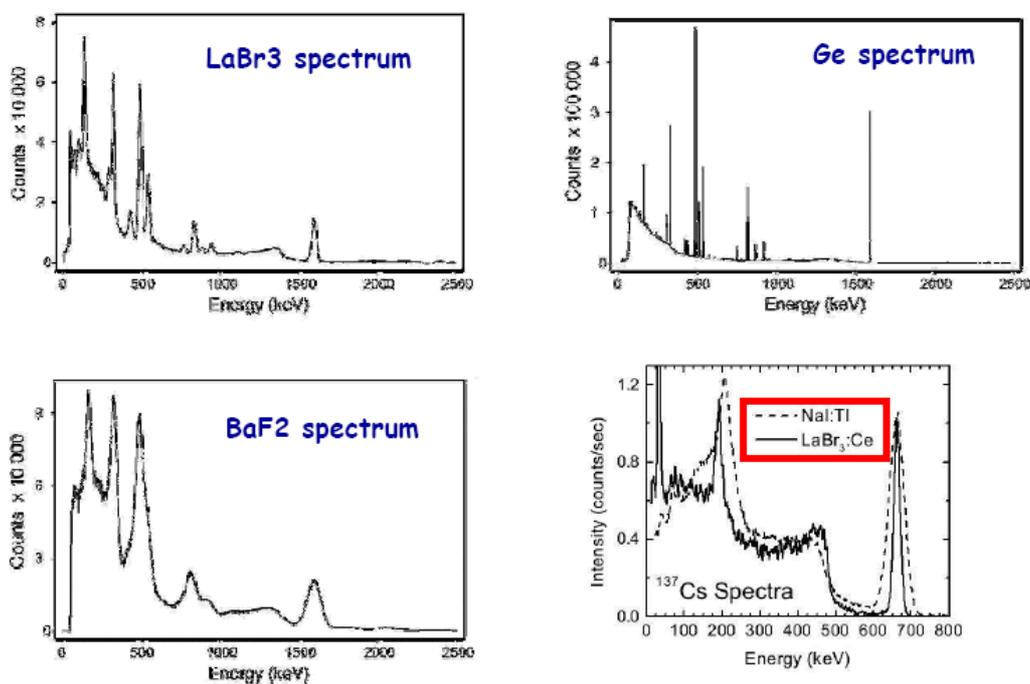
**Figure 34:** Comparison of different energy spectra used in fast-timing experiments. The improvement in energy resolution when  $\text{LaBr}_3$  scintillators are used, instead of  $\text{BaF}_2$ , is clearly visible.
