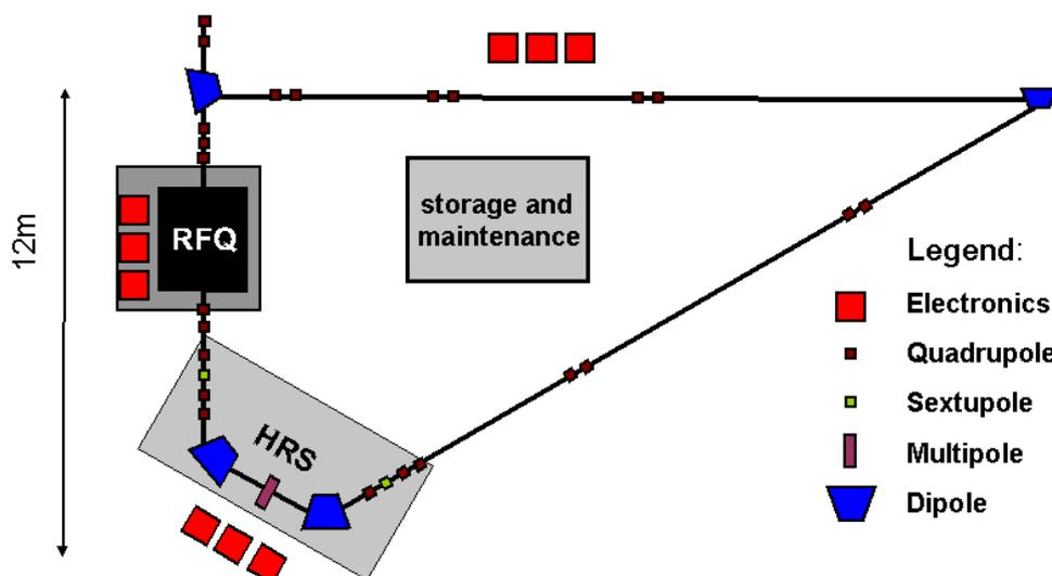
*Figure 4: Layout of the RFQ-HRS room in the SPIRAL2 production building. A beam line bypassing the RFQ and the HRS is also foreseen.*
