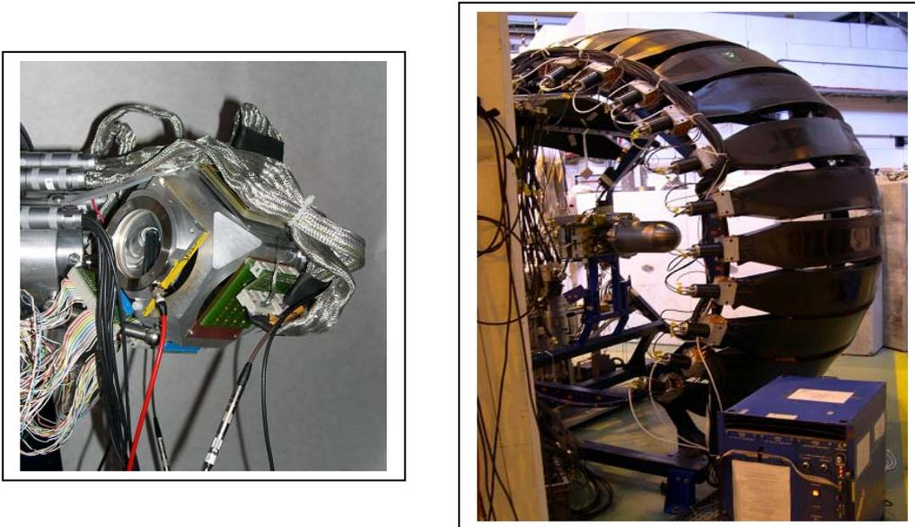
**Figure 36:** A typical decay spectroscopy experiment. The TONNERRE neutron ToF detector is surrounding a charge particle setup (on the left) for studying  $^{11}\text{Li}$   $\beta$  decay at ISOLDE.
