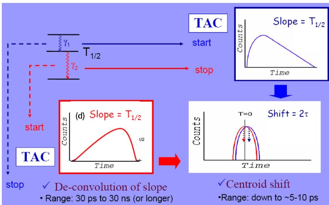
Figure 33: Different time spectra obtained for different gating conditions and different lifetimes.
