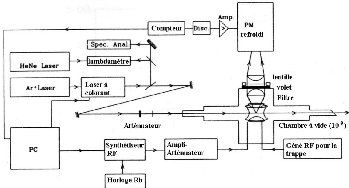
Figure 21: Complete radio-frequency setup with its Paul trap (from [Bec93]).
