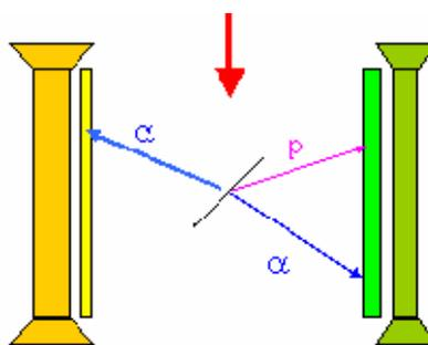
**Figure 35:** Typical experimental setup in decay experiments. Highly segmented Si detectors surrounding a thin C-foil where the radioactive source is deposited. The segmented detector is stacked with a thick Si-PAD detector to act as a  $\Delta E$ -E telescope in order to detect and distinguish between particles of higher energy and/or  $\beta$  particles.
