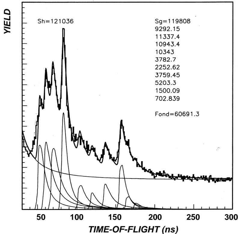
**Figure 30:** Neutron TOF spectrum for the  $\beta$ -delayed neutron decay of  $^{46}\text{Cl}$  obtained by S. Grévy and collaborators using the TONNERRE array.
