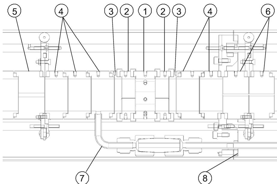
**Figure 42:** *Electrode structure of the purification trap: (1) eight-fold segmented ring electrode, (2) 2-fold segmented first correction ring, (3) second correction ring, (4) end caps, (5) diaphragm at injection side, (6) diaphragm between the traps (two parts), (7) gas-feeding line to the purification trap, (8) pumping barrier between the two traps.*
