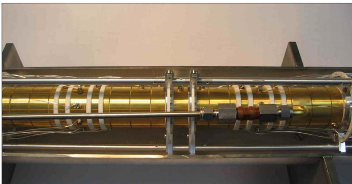
**Figure 44:** Photograph of the electrode system of the double Penning trap system of MLLTRAP.
