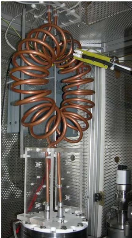
**Figure 9:** *RF high voltage transformer:
