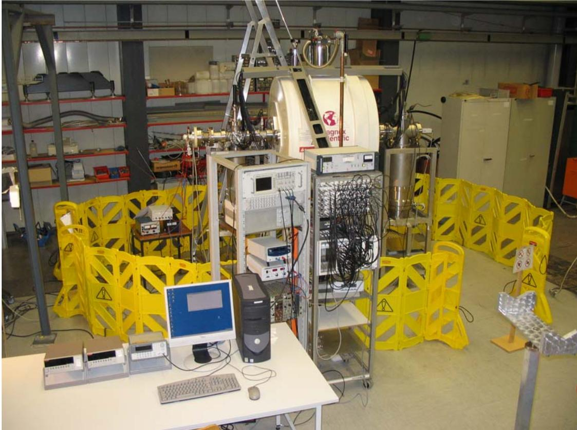
*Figure 40: View of the MLLTRAP Penning trap setup as presently commissioned at the Maier-Leibnitz-Laboratory in Garching/Germany.*
