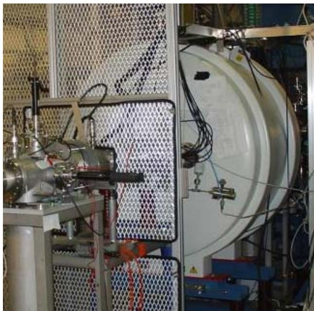
*Figure 26: The superconducting magnet of the JYFLTRAP system at Jyväskylä is shown as mounted at the IGISOL facility. The double trap system is housed in the centre of the magnet. In the foreground, the extraction beam line is visible [IGISOL].*
