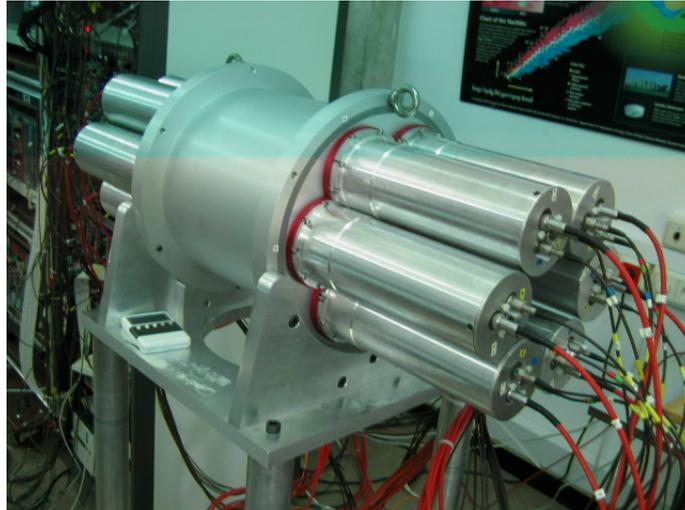
**Figure 23:** *The BaF<sub>2</sub> Total Absorption Spectrometer.*
