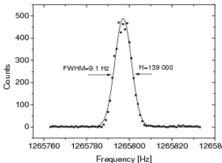
**Figure 45:** Frequency scan in quadrupole mode for the determination of the cyclotron frequency  $f_c = 1265797.11(6)$  Hz for  $^{85}\text{Rb}$  in the purification Penning trap, resulting in a mass resolving power of  $R = 139(2) \cdot 10^3$ . Black dots in the plot are the measured data points and the black line is a Gaussian fit with a width of 9.10(15) Hz (FWHM) [kolhinen2008].
