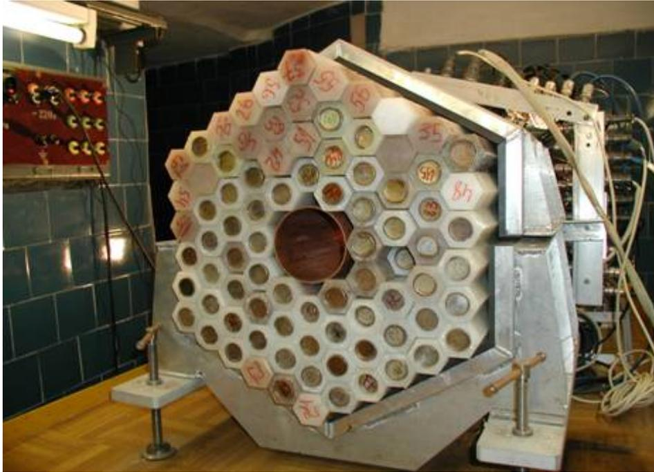
*Figure 29: The neutron detector for the ALTO setup.*
