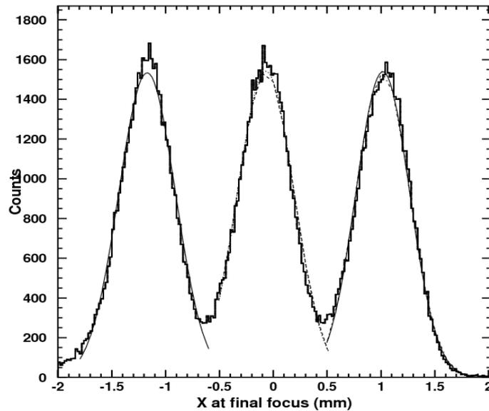
**Figure 13:** Mass separation spectrum as calculated at the final focal plane of the HRS. 50000 particles with mass deviations  $-1/20000$ ,  $0$ , and  $+1/20000$  were transformed through the fifth order transfer matrix.
