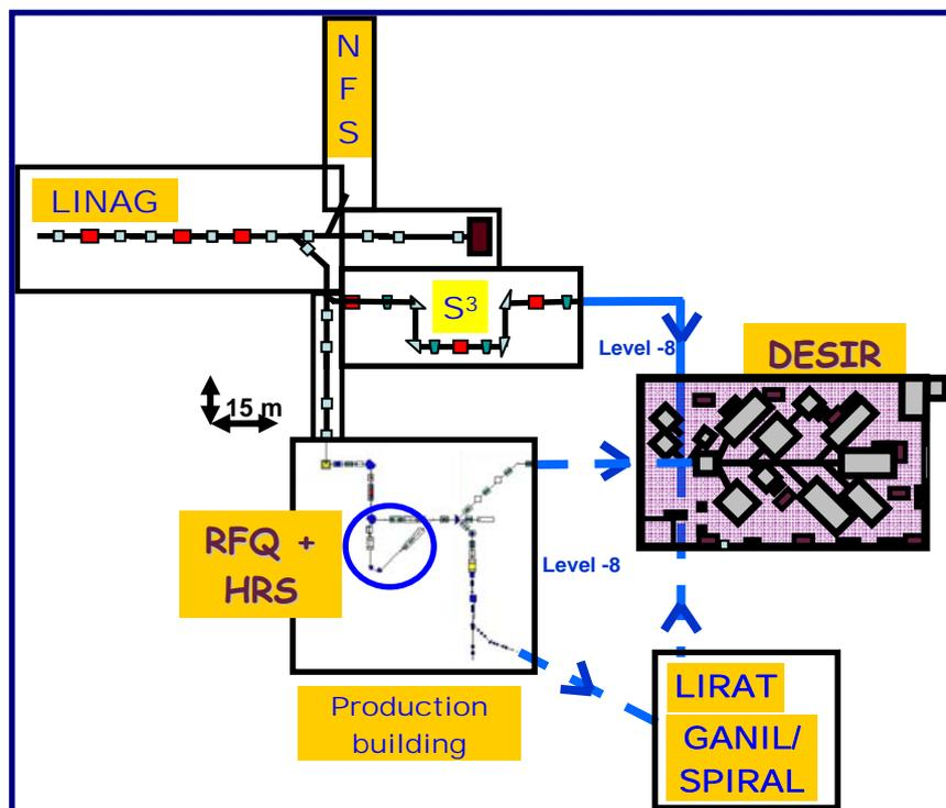
*Figure 2: Schematic layout of the DESIR facility in the GANIL, SPIRAL1 and SPIRAL2 context.*
