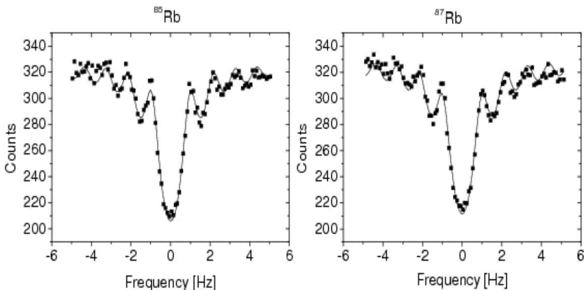
**Figure 46:** An example of frequency scans in quadrupole mode for a determination of the cyclotron frequency with an excitation time of 900 ms. Left:  $^{85}\text{Rb}$ . The frequency axis is scaled such that 0 corresponds to 1266324.354 Hz. Right:  $^{87}\text{Rb}$ . Here the frequency axis is scaled such that 0 corresponds to 1237220.865 Hz. Black dots in the plots are the measured data points and the black lines correspond to the fit functions reflecting the expected line shape [Koe1995].
