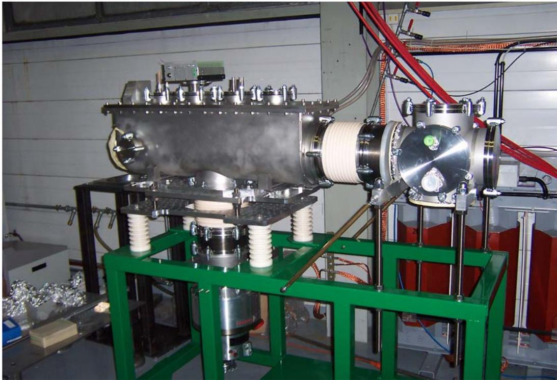
**Figure 18:** Photograph of the ISCOOL buncher now installed after the high-resolution separator at the ISOLDE facility [ISCOOL]. ISCOOL is the first buncher installed on a central beam line to serve different experiments.
