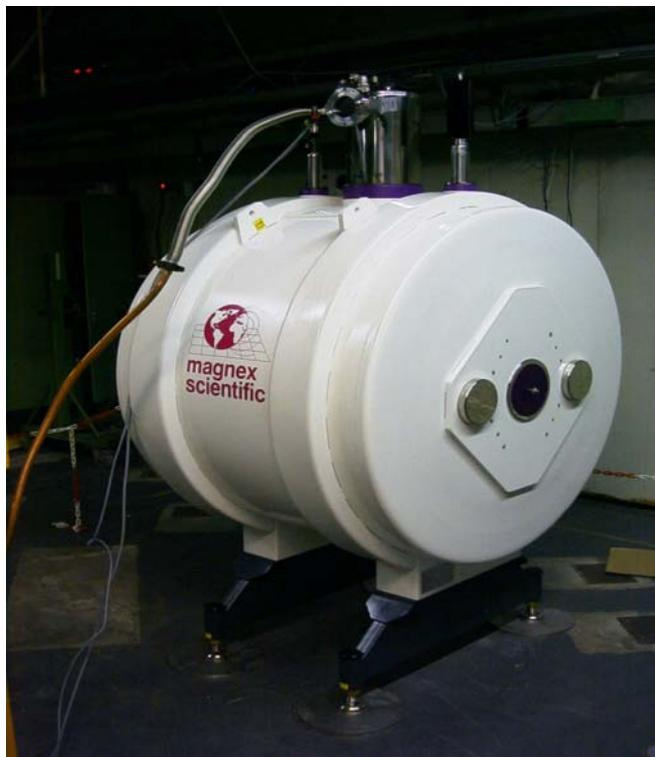
**Figure 43:** *Photograph of the superconducting 7 T trap magnet, forming the backbone of the MLLTRAP double Penning trap facility.*
