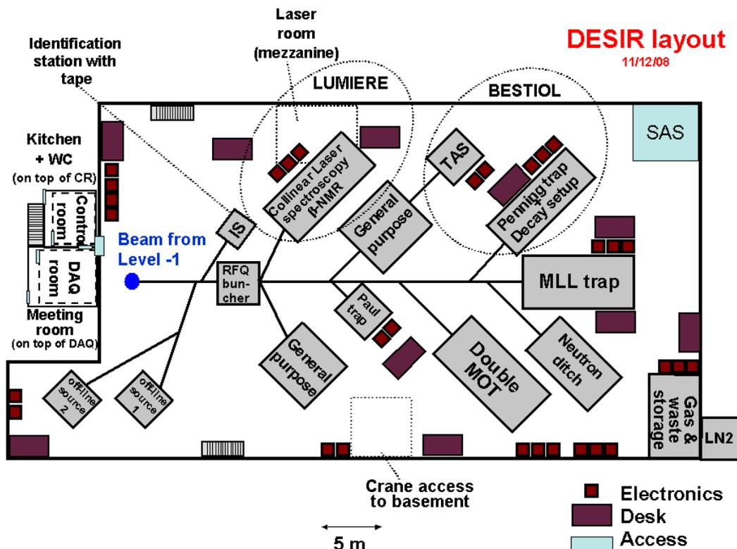
**Figure 6:** General layout of the DESIR experimental hall. The figure shows a possible arrangement of the different permanent installations, the general purpose areas as well as of the meeting, control, DAQ rooms and the kitchen.
