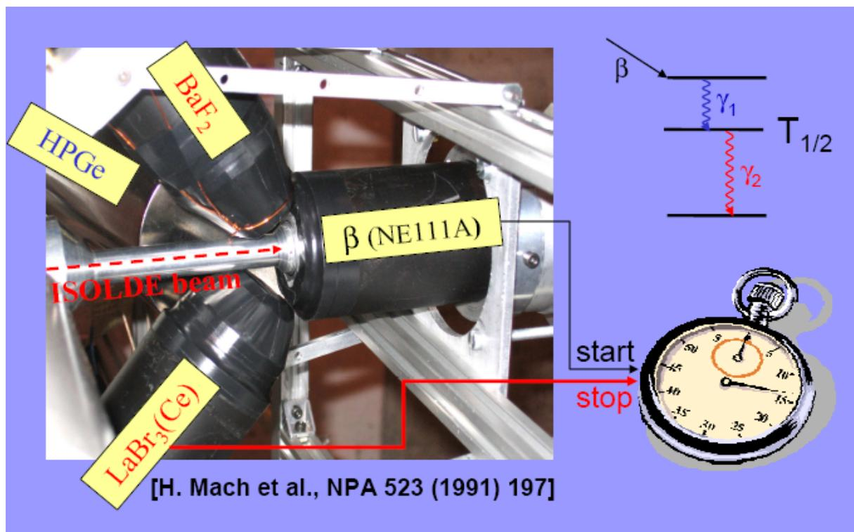
Figure 32: A typical experimental fast-timing setup (ISOLDE). Note one Germanium detector has been removed to allow the other detectors in the setup to be better visualized.
