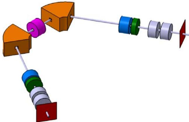
**Figure 11:** 3D layout of the DESIR HRS consisting of two matching quadrupole doublets (grey), two focusing sextupoles (green), two focusing quadrupoles (blue), two 60 degree dipoles and one multipole (pink).
