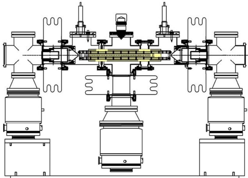
**Figure 16:** Schematic drawing of a general-purpose ion trap, similar to the COLETTE buncher at ISOLDE [COLETTE]. The segmented quadrupole structure is mounted inside
