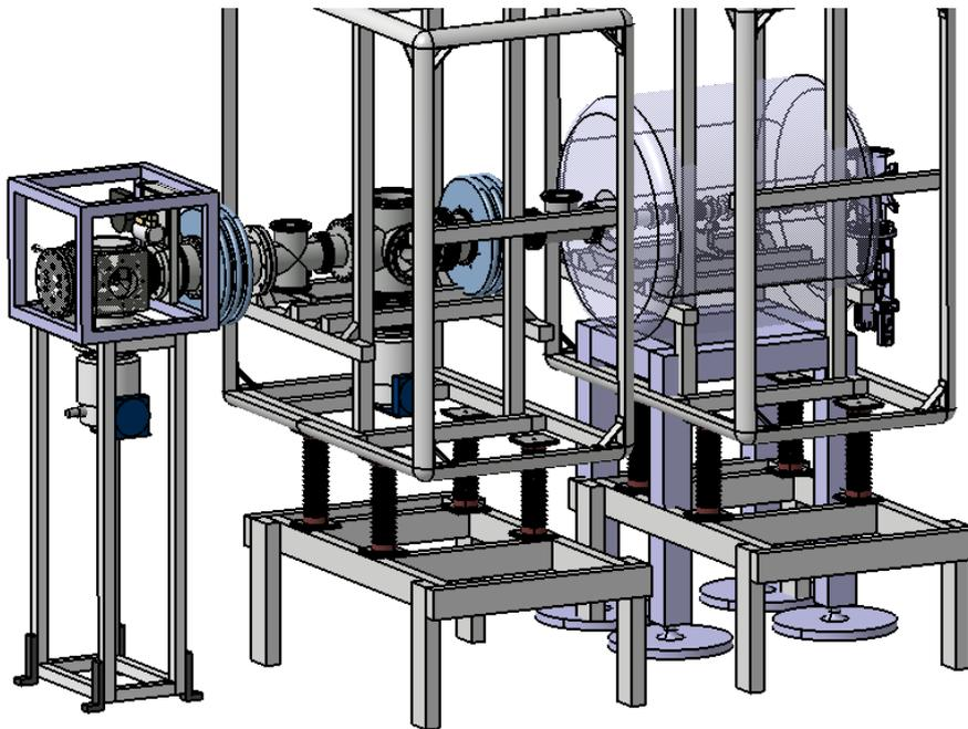
*Figure 24: Schematic drawing of the double Penning trap system.*
