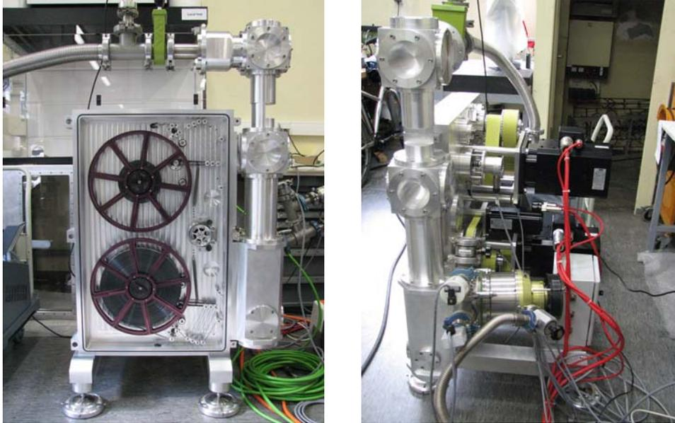
**Figure 15:** General views of an example of a Fast Tape Station equipped with two measuring stations (two cubes with very thin windows) and a device to measure the beam intensity (removal faraday cup).
