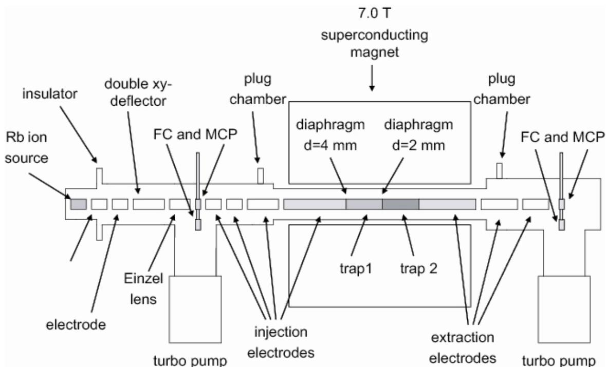
**Figure 41:** Schematic illustration of the layout of the MLLTRAP injection/extraction ion optical system and trap electrodes indicated in the beam line (side view).
